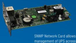
management of UPS across LAN using any of the main network communication protocols - TCP/IP and network interface via SNMP
