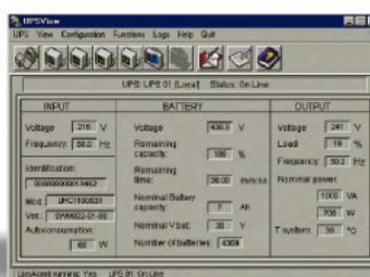
DETAILED UPS PARAMETER DISPLAY Powershield 2 provides all the information required for first level diagnostics.
